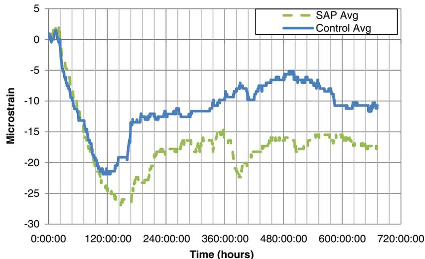
FIGURE 6 Restrained ring shrinkage results (avg = average).
