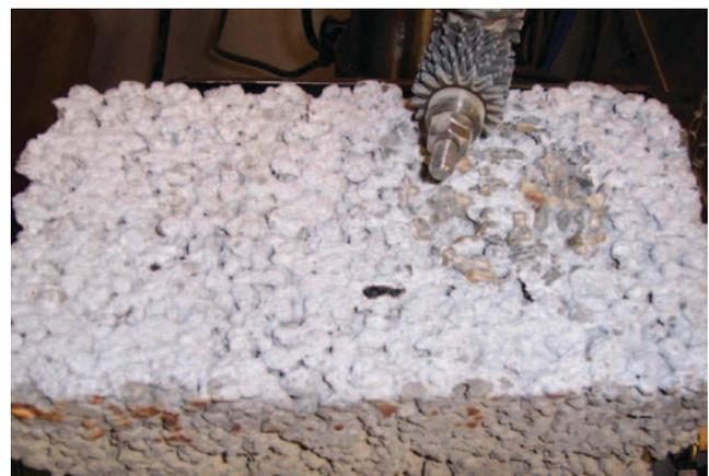
FIGURE 2 Abrasion testing on pervious concrete beam.
