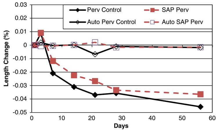
FIGURE 5 Total and autogenous shrinkage results (perv = pervious).
