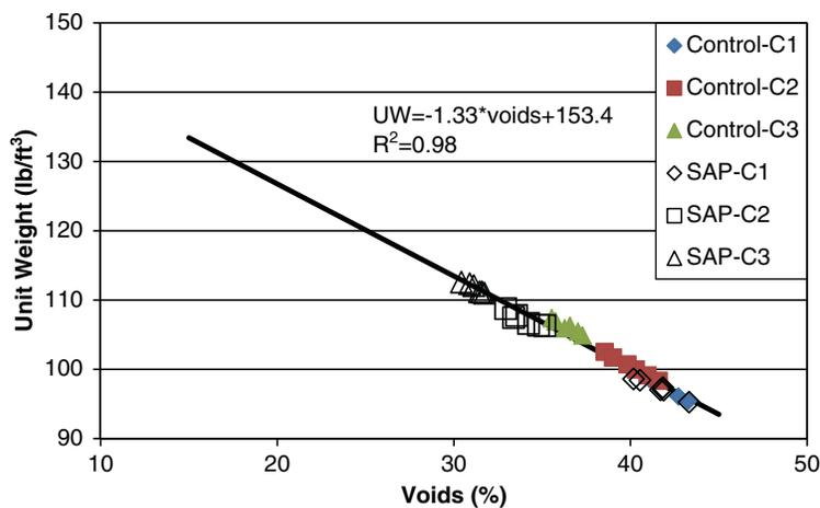
FIGURE 3 Compaction density relationships for mixtures with and without SAP (UW = unit weight).
